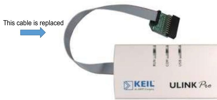
The new cable provided with the ULINKpro unit may have pin 7 filled with a plastic plug. If so, remove the plastic plug before connecting to the Kinetis target. This is easily done with a sharp needle. Merely pry the plastic pin out.
