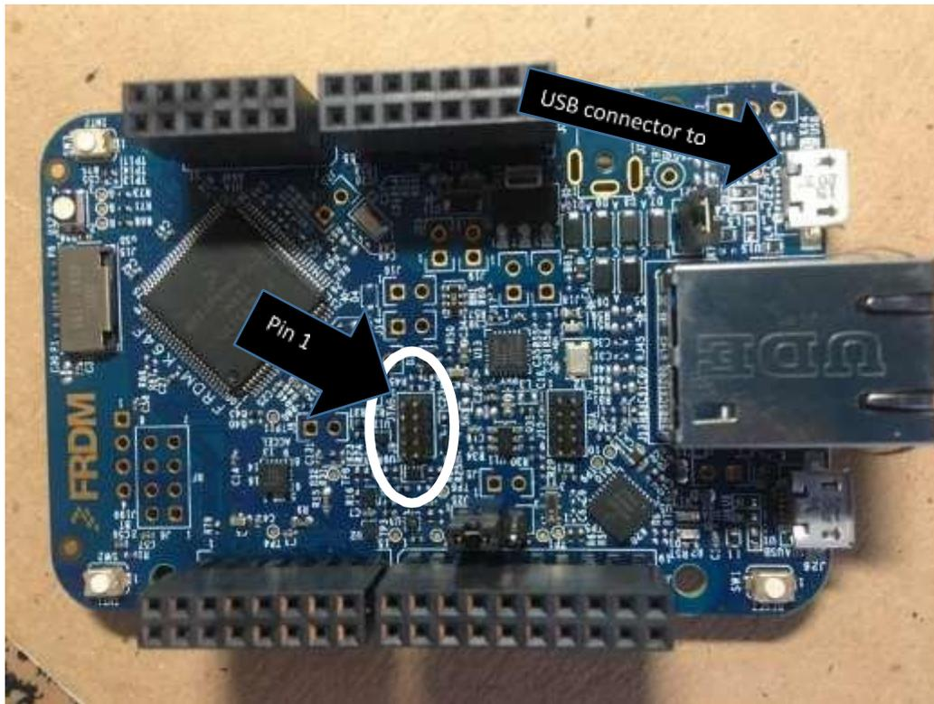
When using OpenSDA, the computer is connected to the SDA-USB port. Ensure this is NOT connected when the ULINKpro is used. Instead, insert the USB cable in the USB port (as shown above). This provides power to the K64F board. Once the JTAG unit is connected to the FRDM-K64F board, install the WNC-Shield board and make the necessary connections (e.g., antenna, power).
