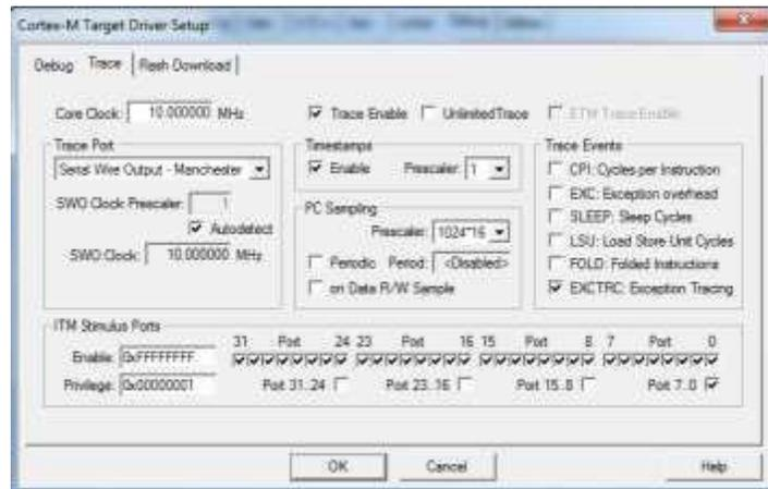
6. Ensure **Port 7.0 and Pin 0** is selected so information can be output to the **Printf (debug)** window. Also verify that **Serial Wire Output – Manchester** is selected. uVision uses Port 0 and 31. All other ports are not used at this time.
