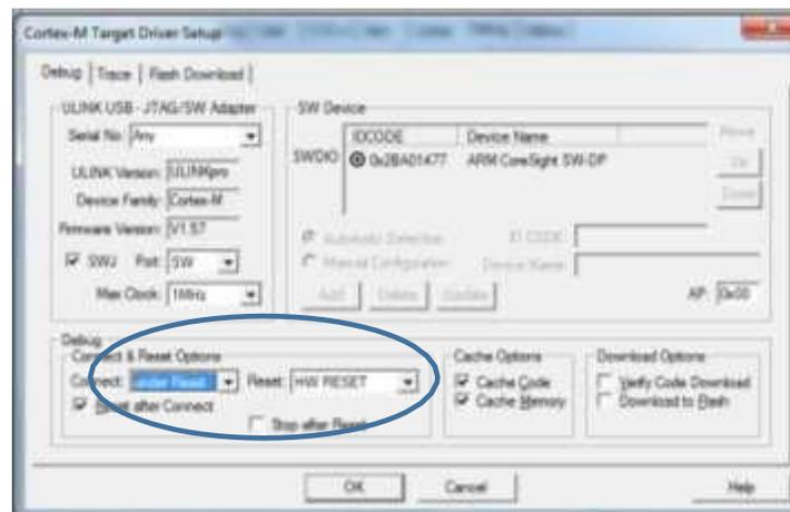
4. Ensure the **Connect & Reset Options** are set as indicated above. That is, **SWJ** is selected and **Port**: is set to **SW**.
