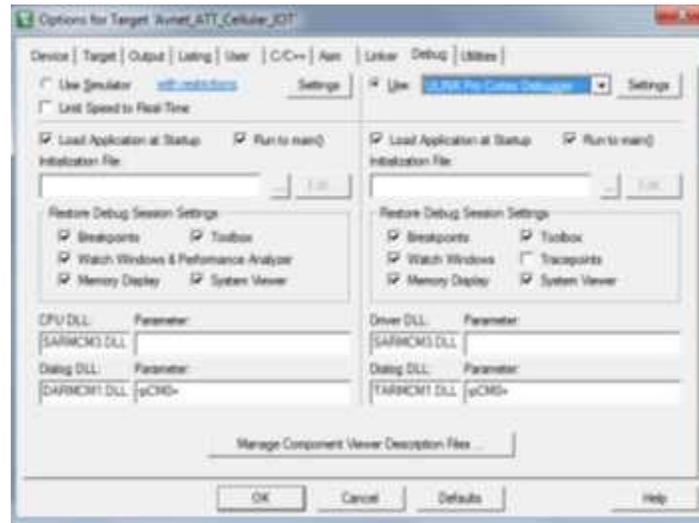
2. From the **Use** selector, choose “ULINKpro Cortex Debugger” (highlighted). The software connects to the ULINKpro debugger.
